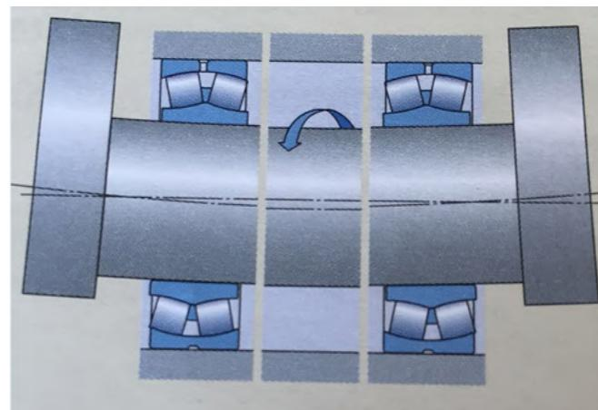
Allow 3 °self-aligning
