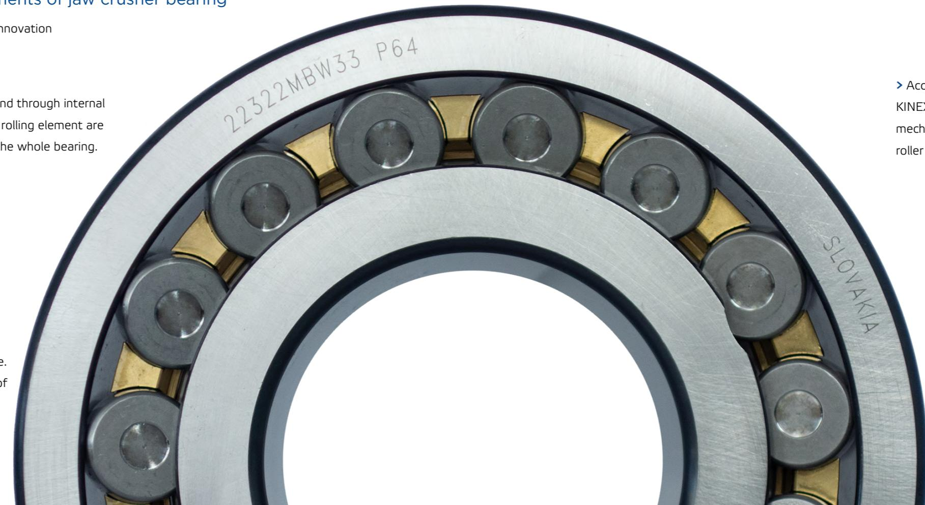
➤ These bearings are designed to withstand high-impact loads, minimize friction, and ensure stable performance in harsh operating environments. The MA-type bearings feature a brass cage, offering enhanced durability and heat resistance, while the MB-type bearings utilize a precision-machined steel cage for superior strength and load-carrying capacity.
